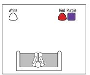
The low-frequency material reproduced by the subwoofer is mostly omnidirectional, and this speaker may be placed in a convenient location in the room. However, the maximum reproduction of bass will be heard when the subwoofer is placed in a corner along the same wall as the front speakers. Experiment with subwoofer placement by temporarily placing the subwoofer in the listening position and moving around the room until the bass reproduction is best. Place the subwoofer in that location.
